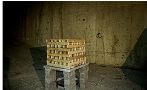
Figure 3: Wood Crib Set up
